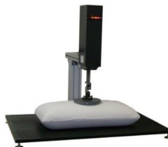
Indentation Load Deflection of Foam products using Model 110-10
