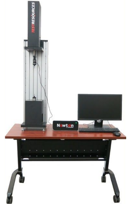
The 131AT frame can be placed horizontally or vertically on a table
